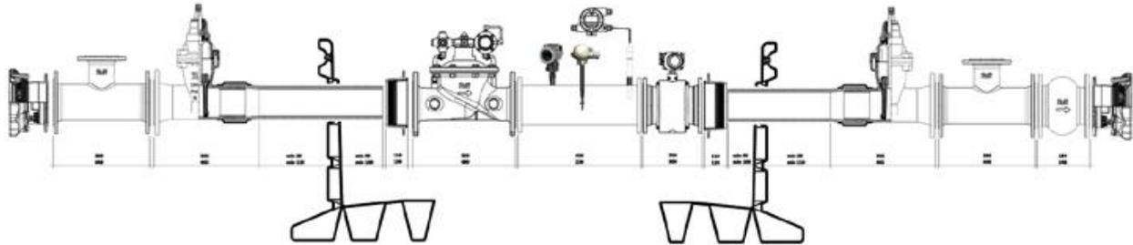
The Pressure & Flow Control and Monitoring Device (PFCMD) is a hydraulic control valve with one or more control functions as per the requirements such as
